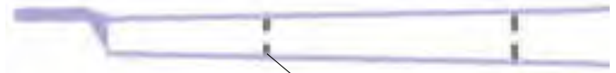
Press-fit the discs into the arm tube using a threaded rod and nuts as shown below
