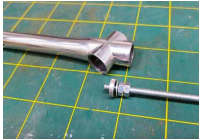
The best tool for fitting the bracing discs is a length of M4 (or 3/16 unf) threaded rod with two nuts locked on the end. Use this to tap the discs into place.
