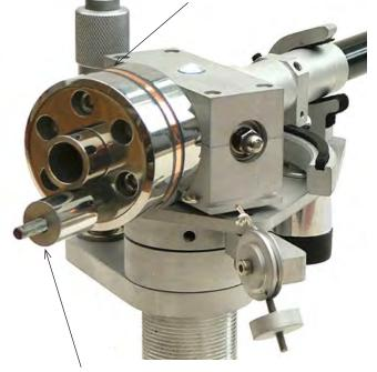
The fine adjustment weight goes at the bottom. Approximately set the tracking weight (VTF) by moving the large weight, then adjust it to the final setting with the small weight.
