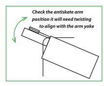
Before mounting the arm, check the position of the antiskate arm. It is shipped turned towards the back to avoid damage in transit.. Twist the assembly so it aligns with the arm yoke when the tonearm is in the arm rest. Make final adjustment later. **Set the**
