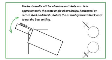
Ser the weight towards the top for MM cartridges start here for MC cartridges
