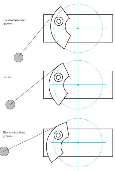
Turn the antiskate arm to a position where the thread sits in the groove of the quadrant.
