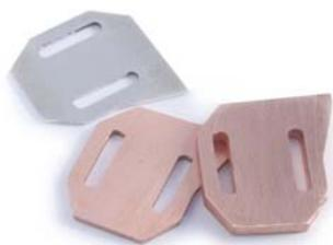
*Mass shims are supplied with Series Five arms and are used with many moving coil cartridges to tune the response. Use the lighter one for the 301, the 10g shim for the 103.*
