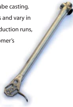
Constrained layer counterweight with lead damping and secondary weight for fine vtf adjustment.
