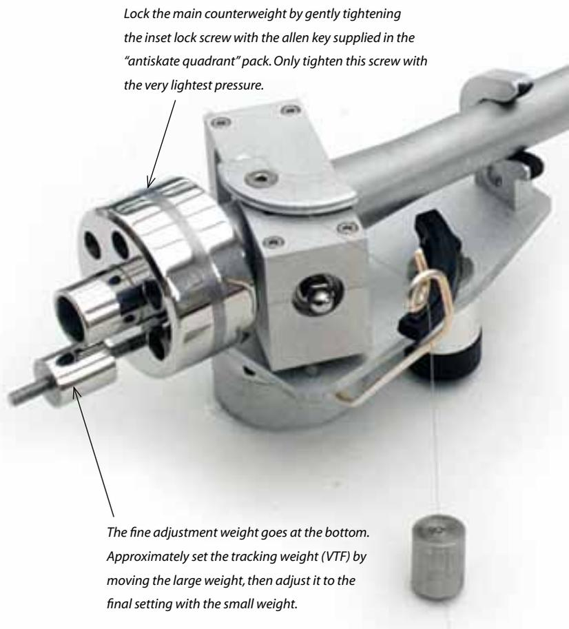
Lock the main counterweight by gently tightening the inset lock screw with the allen key supplied in the "antiskate quadrant" pack. Only tighten this screw with the very lightest pressure.
