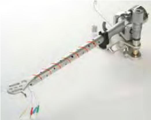
Take the printed drilling template and cut it into two strips. Join the ends A-A to make one long strip. This is much longer than you will actually need.
