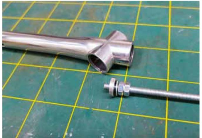
*The best tool for fitting the bracing discs is a length of M4 (or 3/16 unf) threaded rod with two nuts locked on the end. Use this to tap the discs into place.*
